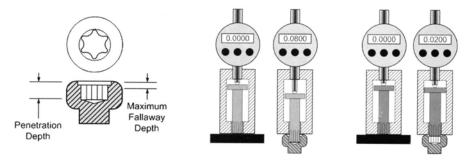
The 6 Lobe recess is one of the most popular fastener recess designs throughout the world for high volume fastener assembly applications. This recess design is particularly popular where consistent fastener tightness is critical to the quality and performance of the end product.
